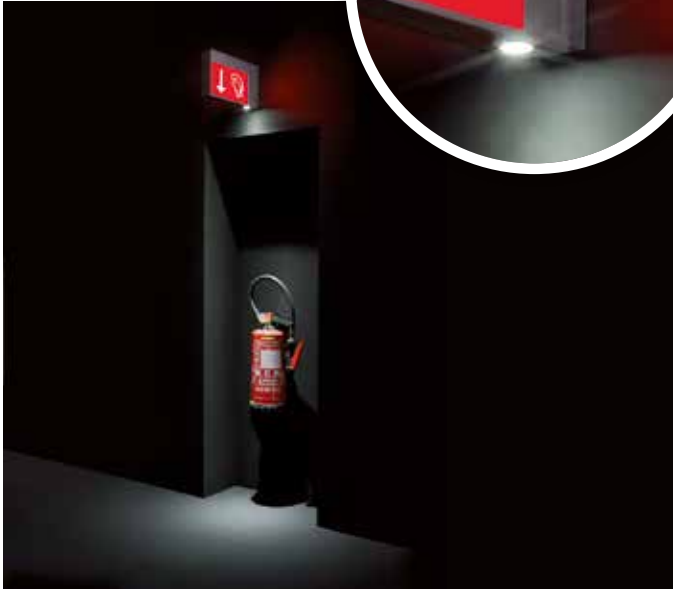
With a light spot module 5 lux is achieved, up to 4 metres mounting height without extra luminaires.
